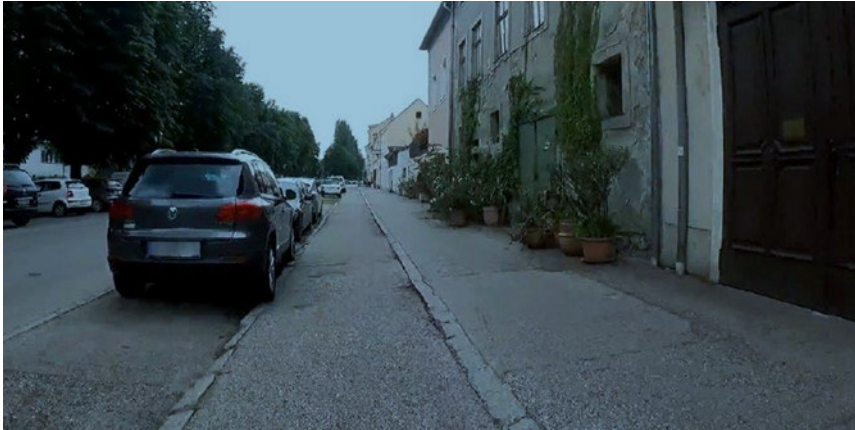
Figure 34 Curb-side parked cars too near to bicycle infrastructure, Austria. Source: SABRINA (2022, copyright @EuroRAP)
